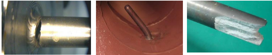
Figure 2. Examples of Thermowell Failure
