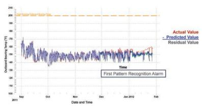
Predictions of imminent failures are valuable and necessary, and "smart" technology automatically predicts the likely imminent failures. The above left-hand image shows the typical historical trend group which does not clearly show an emerging failure condition; the same data is shown in the right-hand image, where the smart pattern recogniser accurately identifies the emerging condition and make the visualisation clear, with associated notifications and alerts.
