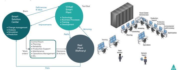
The previous diagram shows the main data flows between the physical refinery, the main Refining Operations Management system in an Operations Center, and the virtual Refining Operations Management system. The notifications and instructions from Refining Operations Management aren't formal work orders, but they are a set of information, instructions and notifications which are used by professionals, technicians and field workers.
