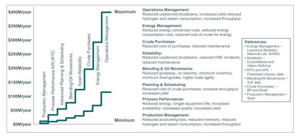
To achieve and sustain this level of performance, the refinery needs to operate differently. This type of operation is often called the Smart Plant. The refinery isn't "smart" because it has more sensors, more data or more computers; it is "smart" because it operates in a "smart" manner, which means that undesired events are prevented more frequently and desired opportunities are "exploited" or taken full advantage of more often.
