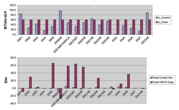
The above report shows a profit analysis and efficiency benchmarking of 17 heat exchangers. This is a good example of proactive information- all of the heat exchangers are serviceable, but limiting the duty of a crude unit fired heater reveals the sensitivity to economic performance of at least one of these heat exchangers. This is much more than predicting imminent failures or corrosion analysis.
